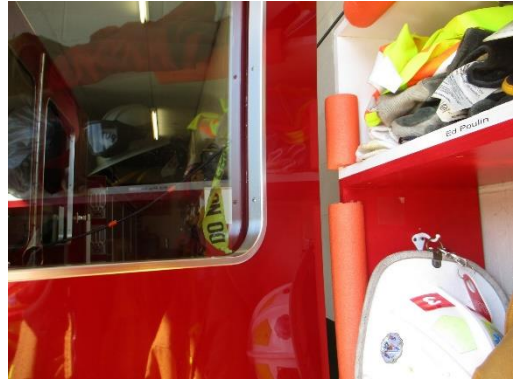
08 – Door protectors needed on gear lockers
